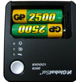
3. Once the batteries are in place, the cover can be re-installed.
