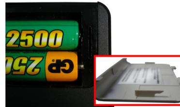
4. With all tabs carefully aligned, hold the DG-100 as shown and apply pressure on the bottom of the cover to slide it and lock it into place.
