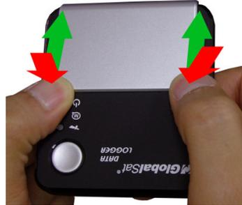
2. Insert the two included “AA” NiHi batteries into the DG-100 in the orientation as shown to the right.
